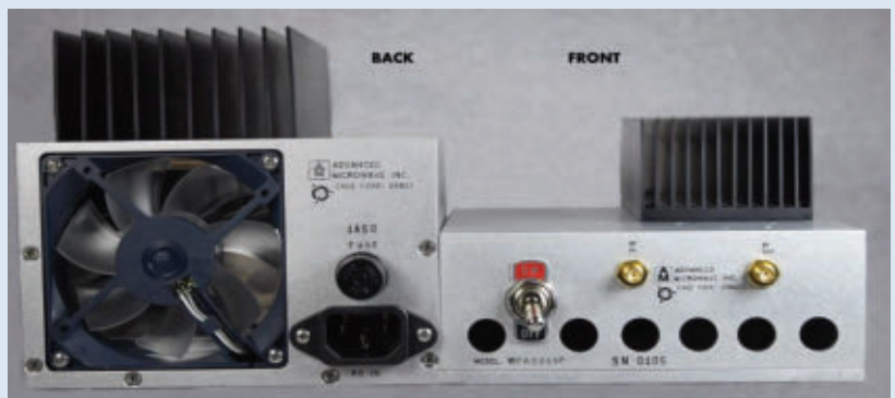
A complete package of any amplifier or converter which includes heatsink and 100 to 240 VAC input.
